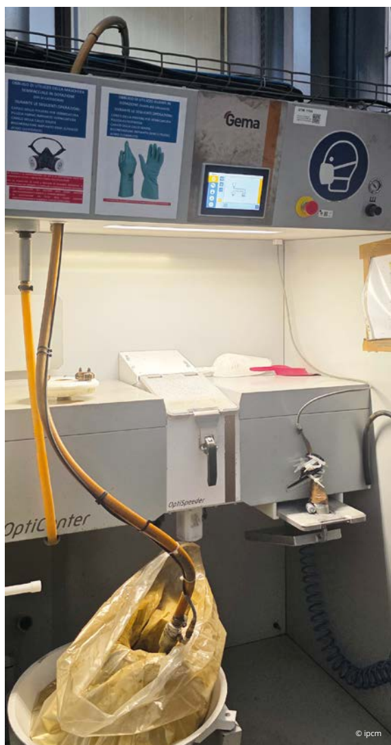
One of the two Optispeeder powder centres WITH Smart-In-Line technology supplied by Gema Europe (Trezano sul Naviglio, Milan, Italy).
