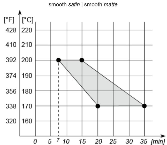
Cure parameters must be closely observed since mechanical properties will develop before full cross-linking.
