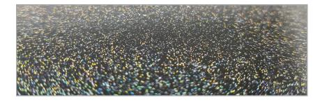
Gold, silver and twilight two-coat glitter powder coating system containing sparkling metallic flakes suspended in a clear top coat applied over a dark basecoat. Astonishing and deep sparkling effects reminiscent of a starry sky, provide the illusion of a fantastic, magical world.
