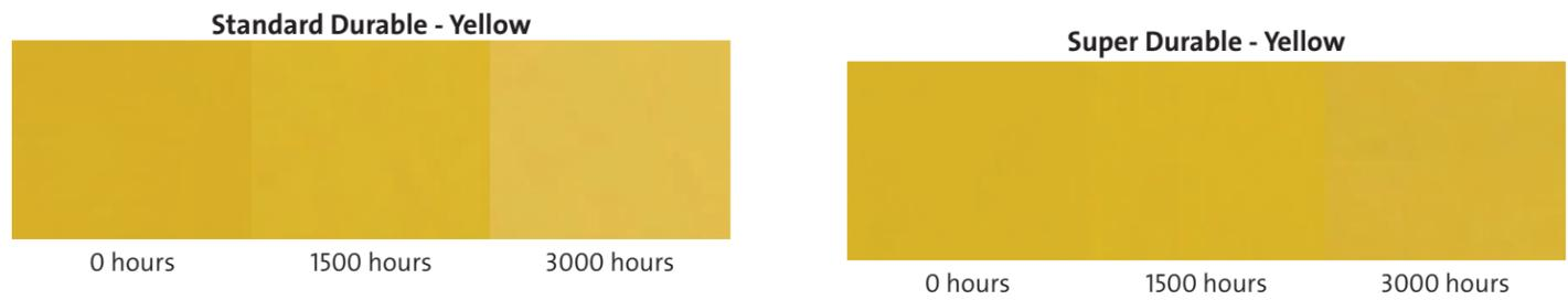
This graph shows how super durable systems fade less than standard durable systems when exposed to south Florida sunlight @ 45° angle facing South. Gloss readings were measured @ 60° angle via ASTM D523.
