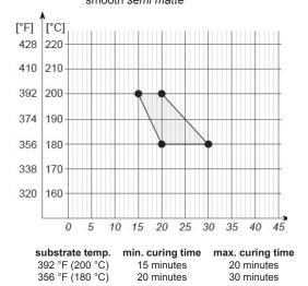
Please observe cure parameters closely since mechanical properties will develop before full cross-linking.
