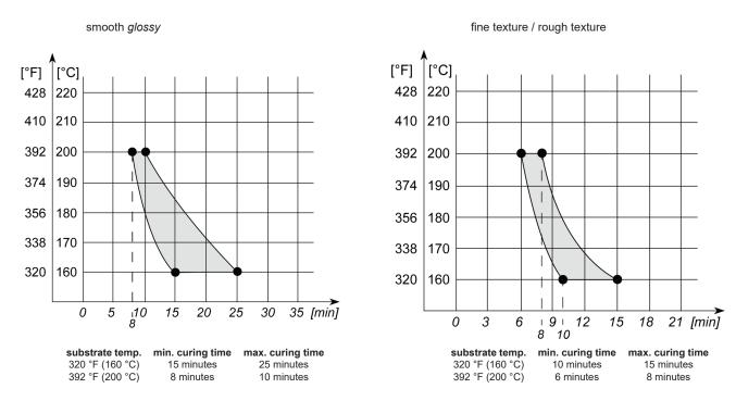
Cure parameters must be closely observed since mechanical properties will develop before full cross-linking.
