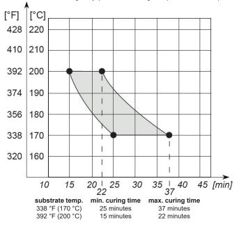
Cure parameters must be closely observed since mechanical properties will develop before full cross-linking.
