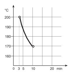
substrate temperature versus curing time
