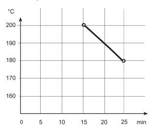
substrate temperature versus curing time
