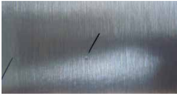
Fig. 3.5.7 Gel particles in powder coating
