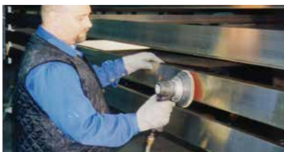
Fig. 3.5.1 Contamination of paint surface from grinding jobs
