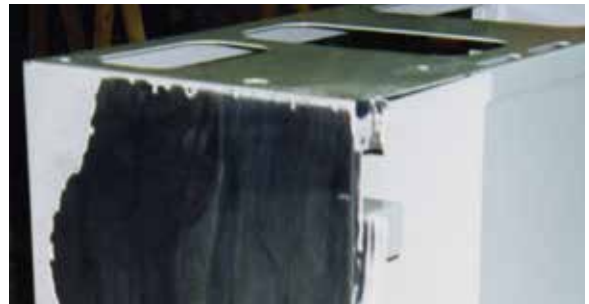
Fig. 2.3.2 Powder film slips off entirely
