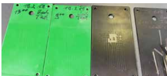
Fig. 1.1.4 Conversion film too thin.
