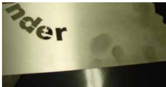
Fig. 3.2.5 Fingerprints beneath clear coat
