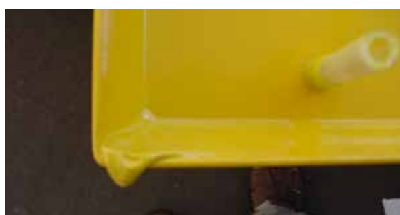
Fig. 3.7.1 Film thickness too high
