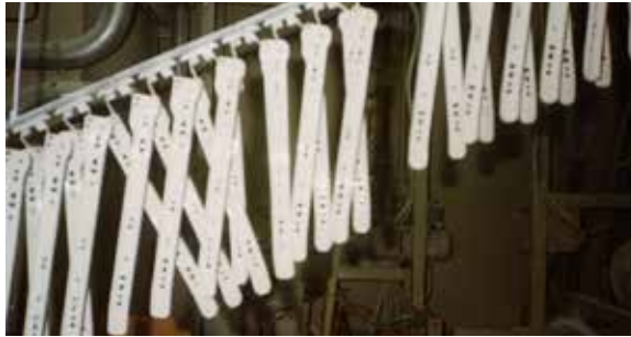
Fig. 2.4.1 Incorrect positioning of workpieces
