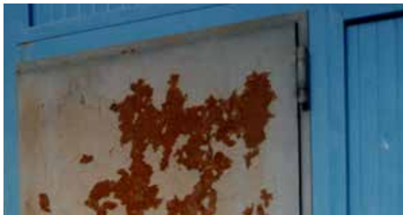
Fig. 5.2.3 Scale, flash rust, white rust
