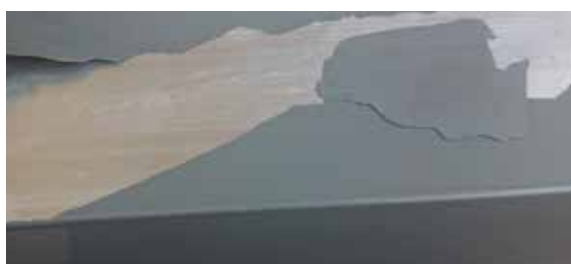
Fig. 1.1.5 Conversion too thick
