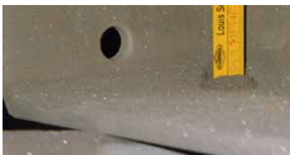
Fig. 2.3.5 Powder film too thick
