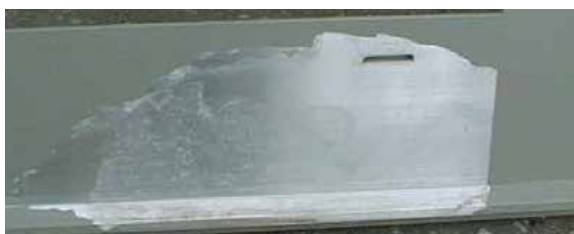
Fig. 1.1.1 Poor (no) chromating
