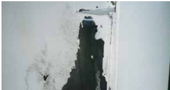
Fig. 2.3.1 Parts of the powder film slip off
