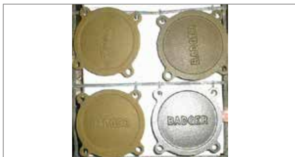
Fig. 1.3.6 Corrosion of sandblasted workpieces after pretreatment
