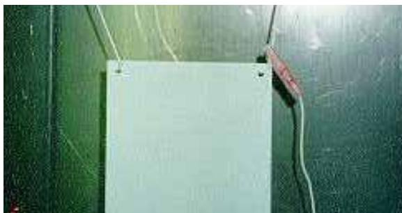
Fig. 2.3.3 No grounding or inefficient grounding
