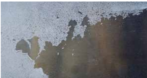
Fig. 3.8.1 Large areas of discontinuity that fail to exhibit a paint film
