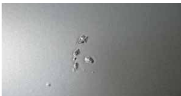
Fig. 3.1.1 Metallic pigment splotches
