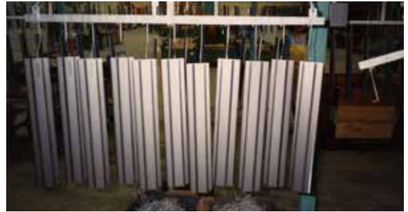
Fig. 2.4.2 Incorrect positioning of workpieces
