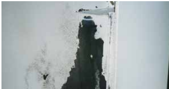
Fig. 2.3.1 Parts of the powder film slip off
