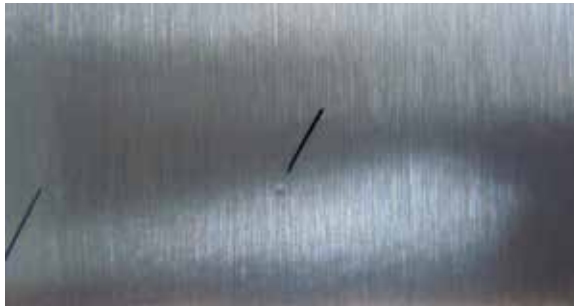
Fig. 3.5.7 Gel particles in powder coating
