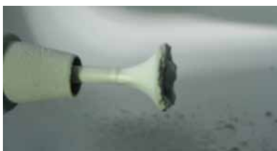
Fig. 2.2.2 Fine particle ratio of powder too high, replace with “Sintering on impact mill”
