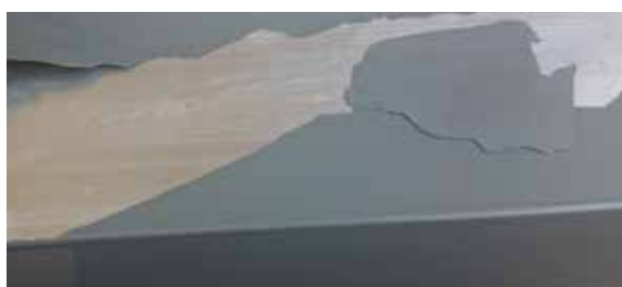
Fig. 1.1.5 Conversion too thick
