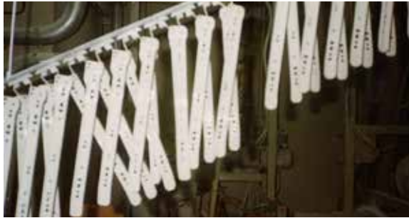
Fig. 2.4.1 Incorrect positioning of workpieces
