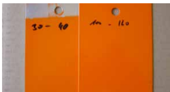
Fig. 4.1.2 Paint films that are too thin and do not cover
