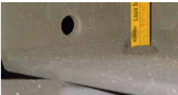
Fig. 2.3.5 Powder film too thick
