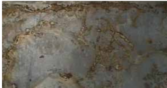
Fig. 1.3.4 Poor rinsing, material stored wet
