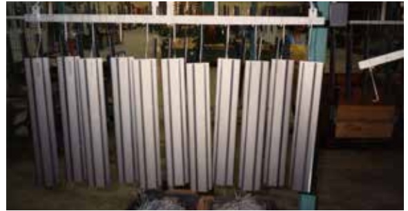
Fig. 2.4.2 Incorrect positioning of workpieces
