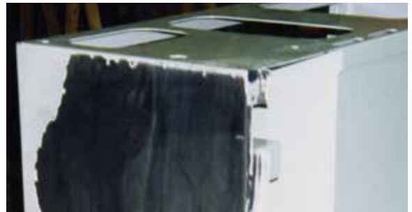
Fig. 2.3.2 Powder film slips off entirely
