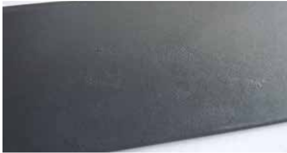
Fig. 3.2.7 Poor rinsing sandblasted, e-coat as base
