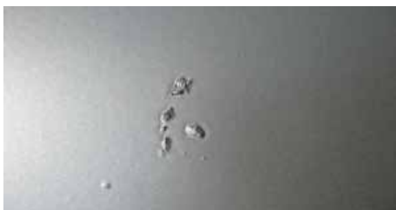
Fig. 3.1.1 Metallic pigment splotches
