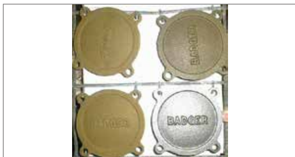
Fig. 1.3.6 Corrosion of sandblasted workpieces after pretreatment
