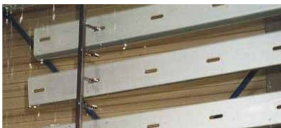
Fig. 1.1.3 Potential transfer of pretreatment media
