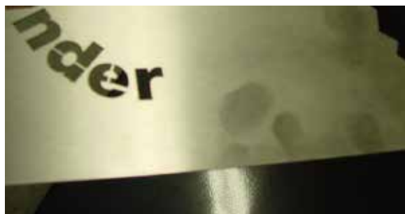
Fig. 3.2.5 Fingerprints beneath clear coat
