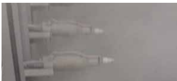
Fig. 2.1.3 Poor fluidization; powder volume too large
