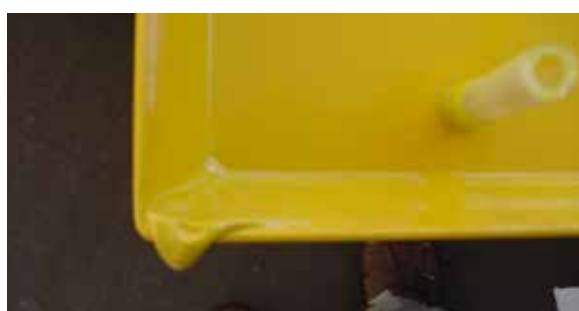
Fig. 3.7.1 Film thickness too high
