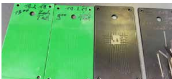
Fig. 1.1.4 Conversion film too thin.
