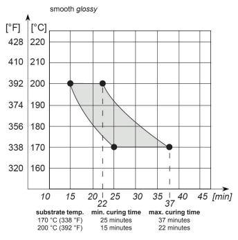
Cure parameters must be closely observed since mechanical properties will develop before full cross-linking.
