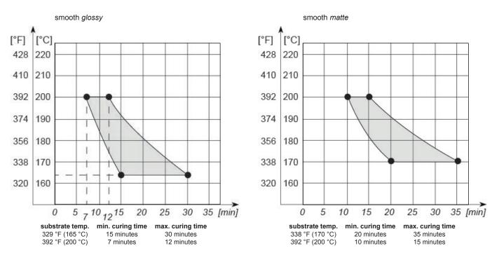
Cure parameters must be closely observed since mechanical properties will develop before full cross-linking.
