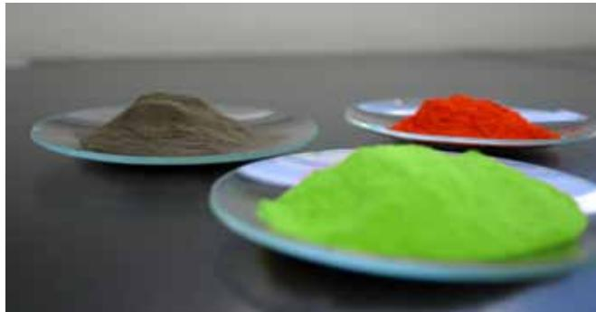
Powder coatings are especially safe for the environment, because they do not release any harmful solvents as they dry. The ability to recycle these powder coatings means that very little material goes to waste.
